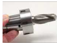
Fully insert cutter into the collet
