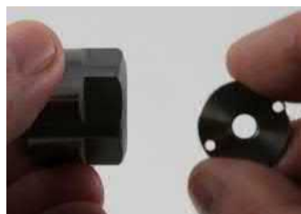
Thread Coolant Cap into SX nut, do not tighten, assemble the collet.
